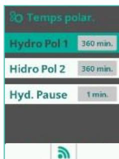
Defines the cycle duration for which the chlorine generation cell runs in polarities 1 and 2 (Hydro Pol1 and Hydro Pos2).
